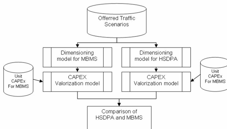
**Figure 4 – Evaluation model for comparing Mobile TV over MBMS and HSDPA.**
