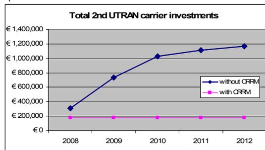
Figure 10 – Total investments needed to support the offered traffic with and without the CRRM algorithm.
