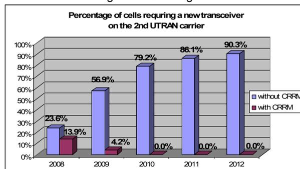
Figure 9 - Percentage of UTRAN cells which require the introduction of new transceivers on the 2nd carrier.
