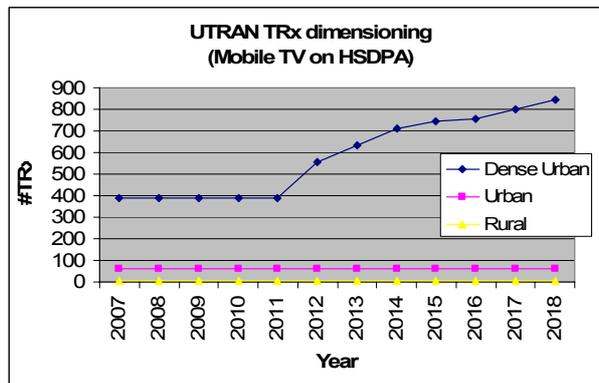
Figure 5 – Transceivers dimensioning (Mobile TV on HSDPA).
